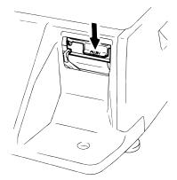
**NOTE:** After replacing the media, press the feed key to confirm that the media is issued correctly. \*Use of other model's label cassette in the SL-9000 may cause a label skew.
